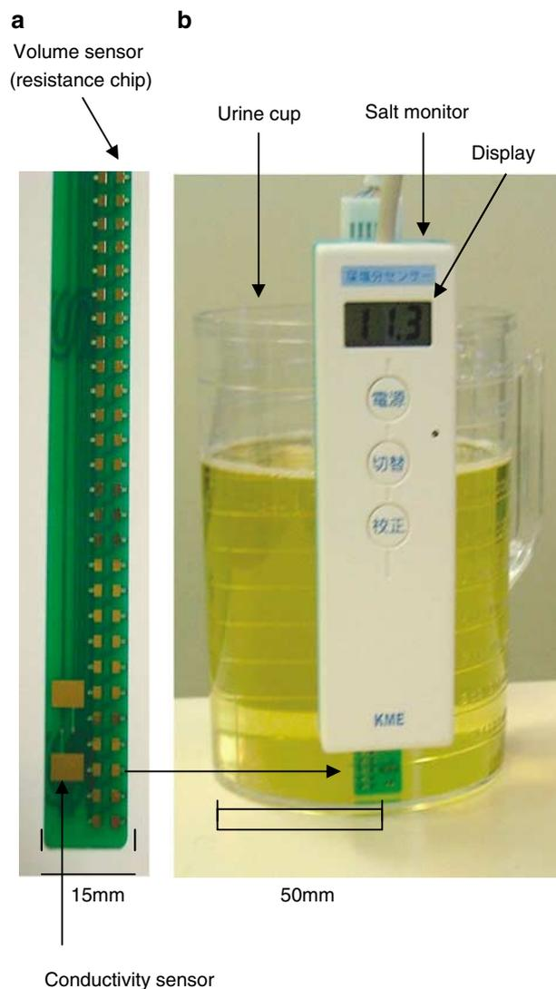
**Figure 1** Salt monitor for estimation of daily salt intake. (a) Conductivity sensor and volume sensor. (b) Salt monitor and urine cup (1-l volume). Daily salt excretion (g/day) is shown on the display.
