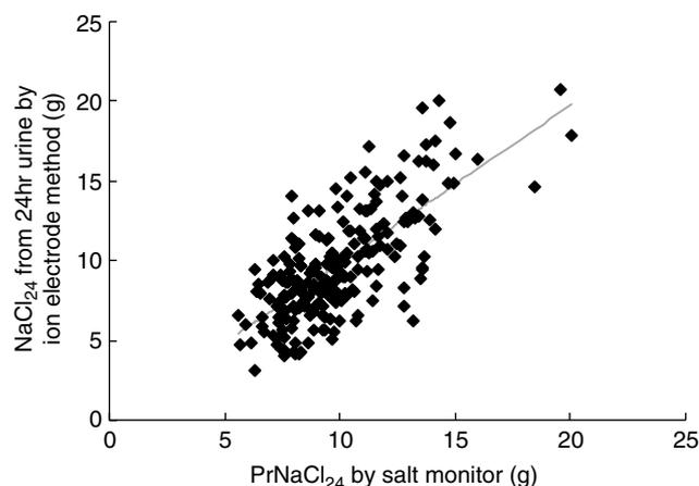
**Figure 2** Relationship between values of 24-h urinary sodium chloride excretion (PrNaCl<sub>24</sub>) predicted from overnight urine by new salt monitor and 24-h urinary sodium chloride excretion (NaCl<sub>24</sub>) by ion electrode method ( $n = 224$ ,  $r = 0.72$ ,  $P < 0.001$ ).
